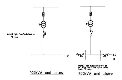
Figure 1: Low Voltage Fusing Arrangements
