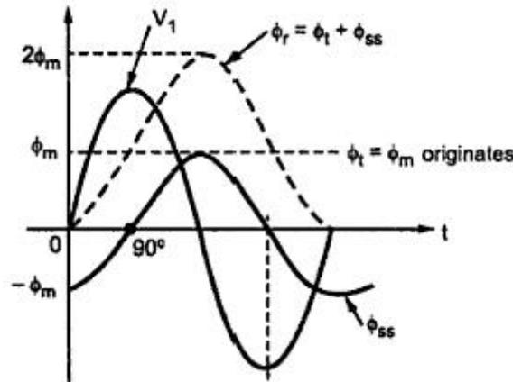
Figure 6- Doubling Effect in a Transformer (Your Electrical Home 2013)
