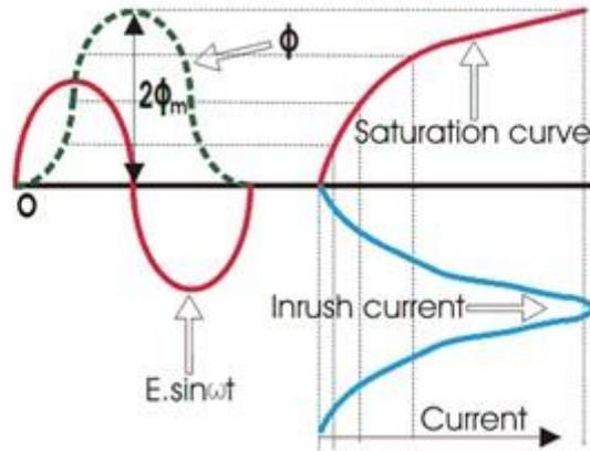
**Figure 5- Inrush Current vs Saturation Curve vs Applied Voltage<sup>7</sup>**
