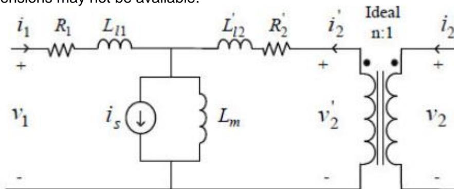
**Figure 2 - Classical Approach - Transformer Model<sup>4</sup>**
