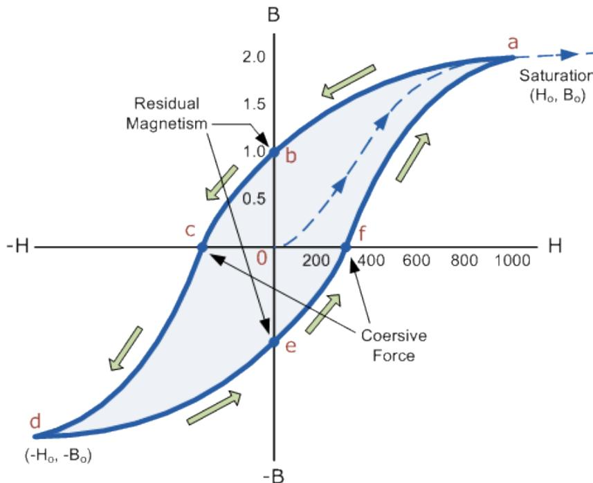
Figure 4- Hysteresis Loop for Magnetism (Electronics Tutorials n.d.)<sup>6</sup>
