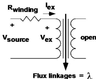
Figure 7- Approximate Transformer Model
