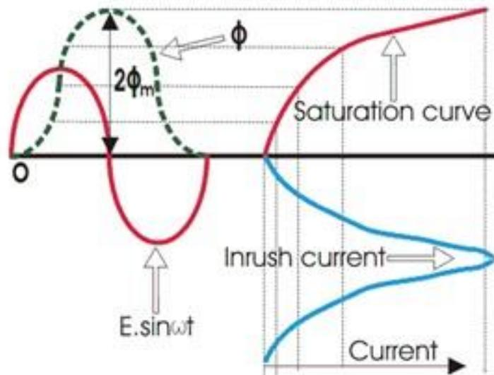
Figure 1 - Inrush Current vs Saturation Curve vs Applied Voltage<sup>3</sup>
