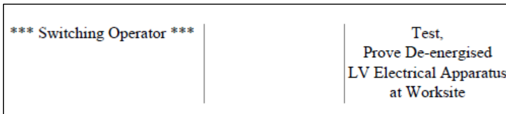
Figure 5 – Example switching Sheet item
